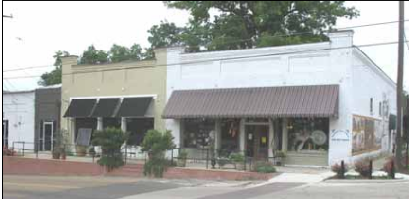
The canvas awnings on these two commercial buildings on Main Street show two appropriate ways to install awnings using a single awning over all of the doors and windows or the alternative of using single awnings over each opening. Originally these buildings had suspended metal canopies.
